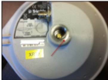
Zephyr-Model 2 Measure Height To: Bottom of antenna mount
